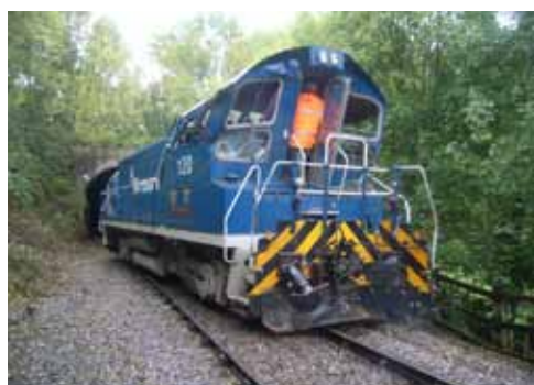
Collision damage to derailed locomotive
