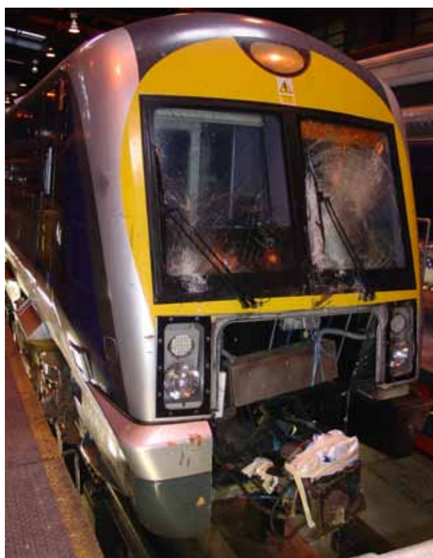
Figure 2: Collision between a train and tractor on crossing XL202 near Limavady Junction, Northern Ireland (Report 10/2008)
