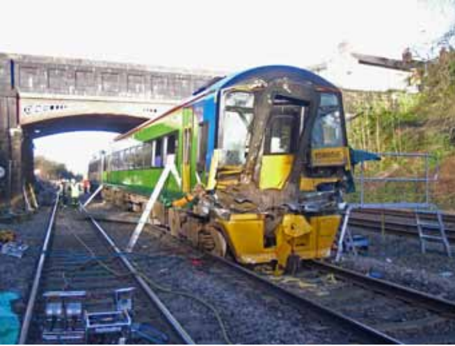
Figure 1: View of the train following collision with the footbridge, Barrow on Soar Report 18/2008.
