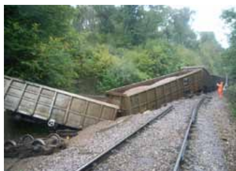
Derailed 3rd, 4th and 5th wagons
