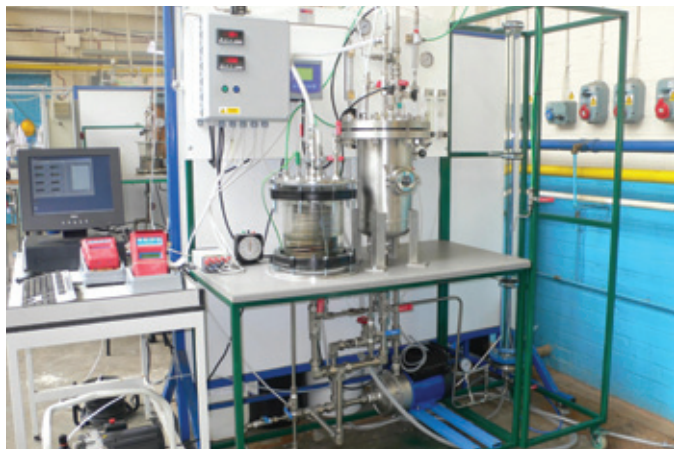
Absorption of CO 2 from air in a DGC reactor - water with sea salt
