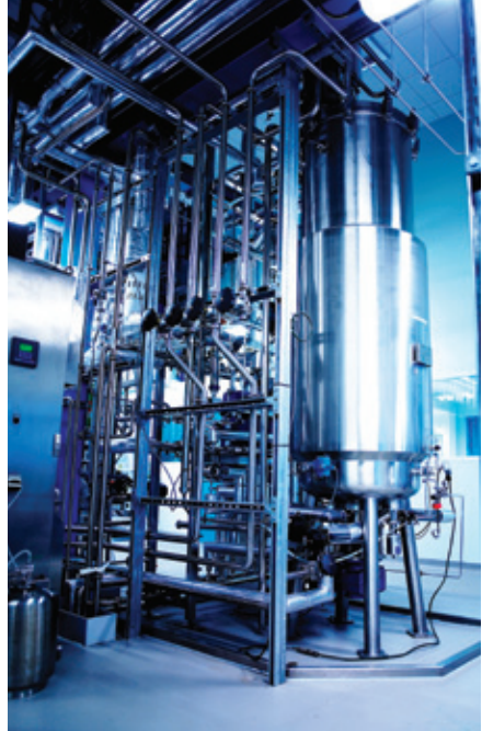
Fermentation vessel used to grow algae samples
