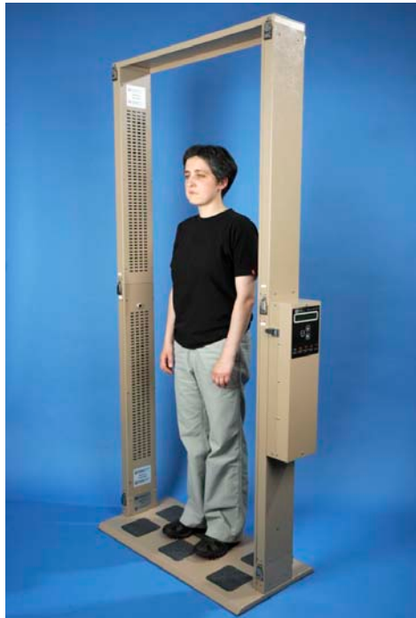
Figure T2. An example portal monitor. The HPA currently have ten in total distributed amongst their centres.
