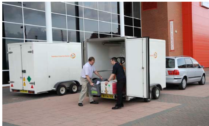
Figure T5. The transportable Whole Body Monitor requires two trailers to deploy.
