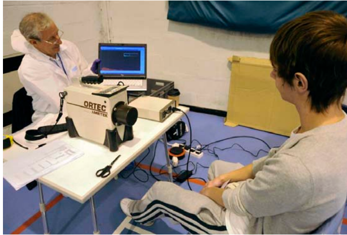
Figure T3. A portable Whole Body Monitor (pWBM) in use during an exercise. The model shown is an Ortec 'Detective'.
