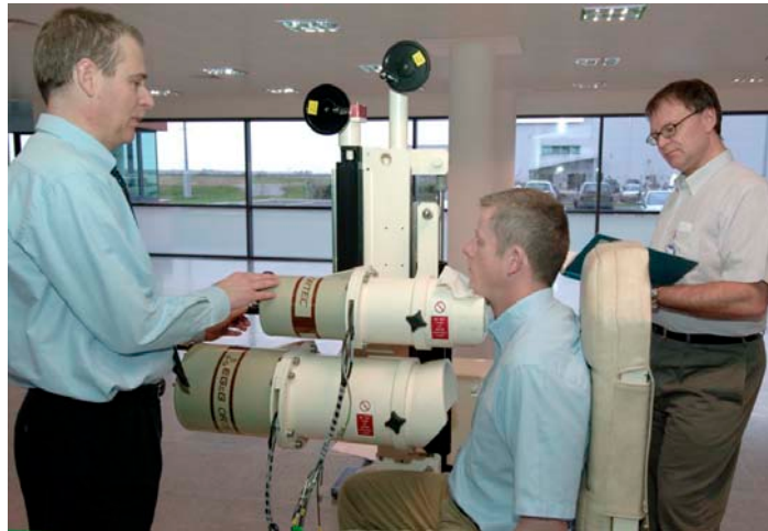
Figure T4. A transportable Whole Body Monitor (tWBM). In use during an exercise. This is a custom made instrument developed by the HPA.
