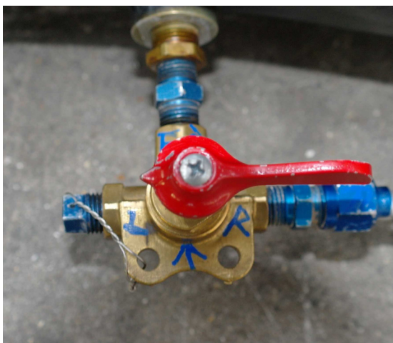
Figure 5 Fuel selector in OFF position
