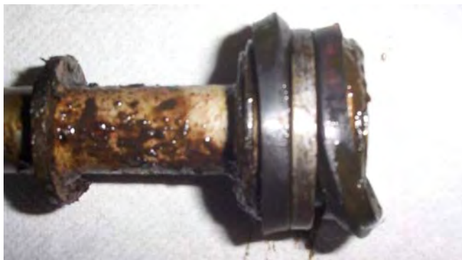
Figure 3 Rolled O-ring seals found on right main gear actuator piston
