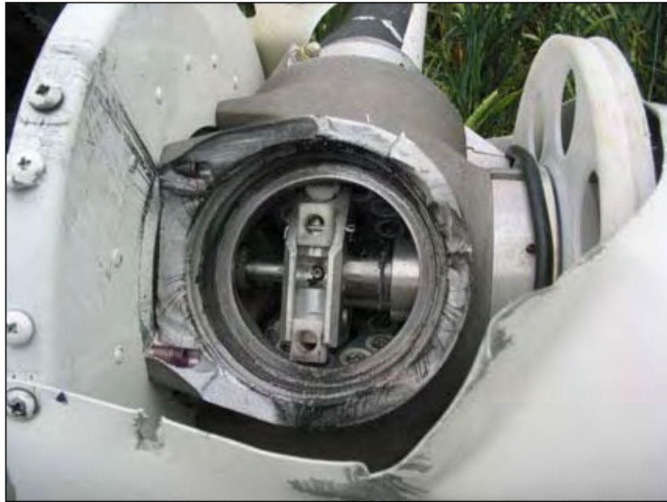
Propeller hub showing fractured No 1 blade socket
