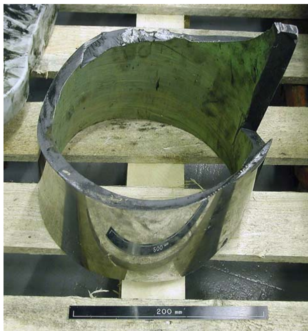
Separated portion of piston Figure 5
