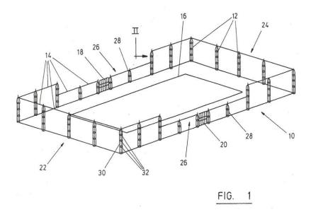
14. As shown in Figures 2 and 3 below, supports 12 may comprise groups of 4 longitudinal members 30 together with associated collars 32 forming a welded structural assembly. The longitudinal members 30 are disposed symmetrically around the collars 32 and are welded thereto. The welded joints are indicated at 38. At the top of each support 12 the longitudinal members may be curved inwards to form generally U-shaped structures which are inter-welded as a structural assembly.
