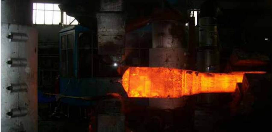
Cogging of rectangular sections for testing.
