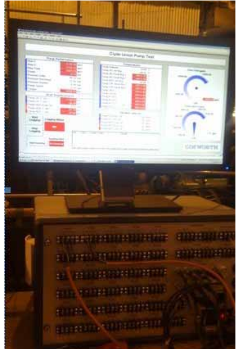
Cosworth real-time data capture system installed on a ClydeUnion pump.
