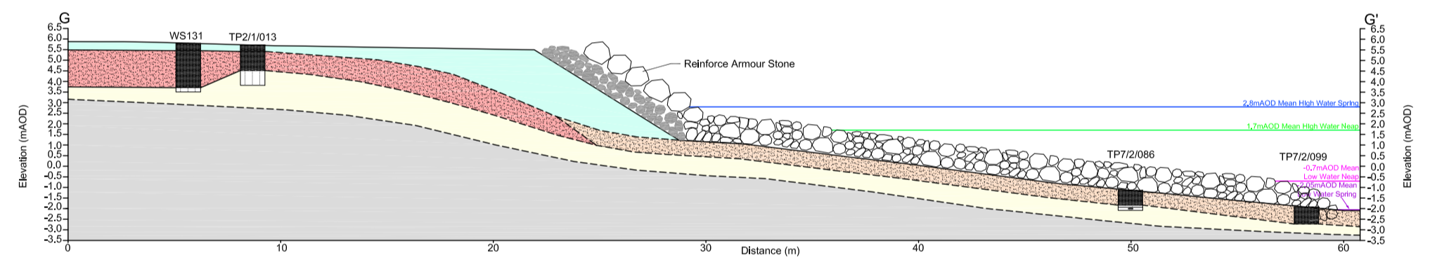
OPTION H4: REINFORCE ARMOUR STONE AND EXTEND ROCK ARMOUR OVER ALL OF FORESHORE SCALE 1:250
