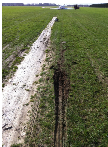
Figure 1 Nosewheel impact mark
