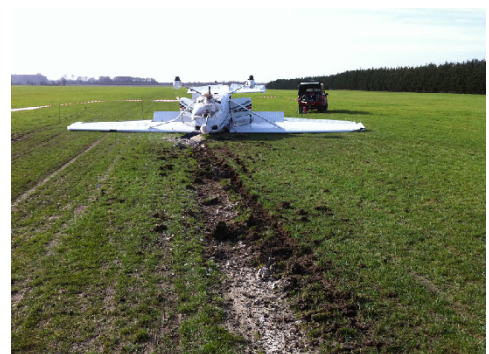
Figure 3 Propeller strike and ground marks
