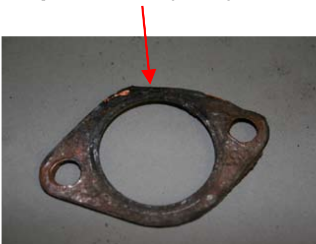
Notable area of carbon deposited which could indicate significant pre-accident exhaust gas leakage
