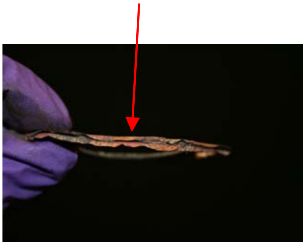
Significant gasket de-lamination
