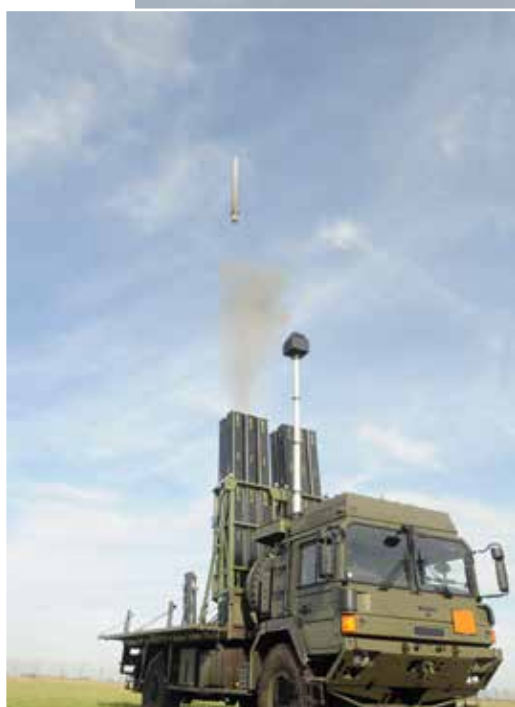
Above: a FLAADS launcher fires a Common Anti-Air Modular Missile during trials. Picture: MBDA
