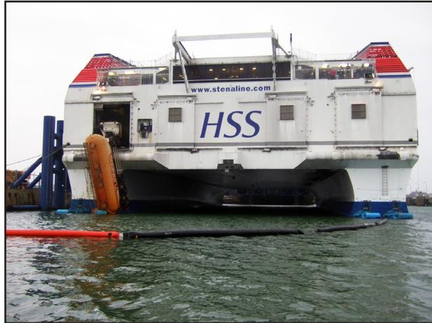
An articulated road tanker crashed through a stern door of the high speed service 1500 (HSS 1500) vessel *Stena Voyager* shortly after the ferry had commenced a scheduled crossing from Stranraer, Scotland to Belfast, Northern Ireland. The vehicle's semi-trailer came to rest on the vessel's port water jet units; its tractor unit remained on the vehicle deck. The ferry was quickly stopped and her crew were able to make the vehicle secure before returning to Stranraer.
