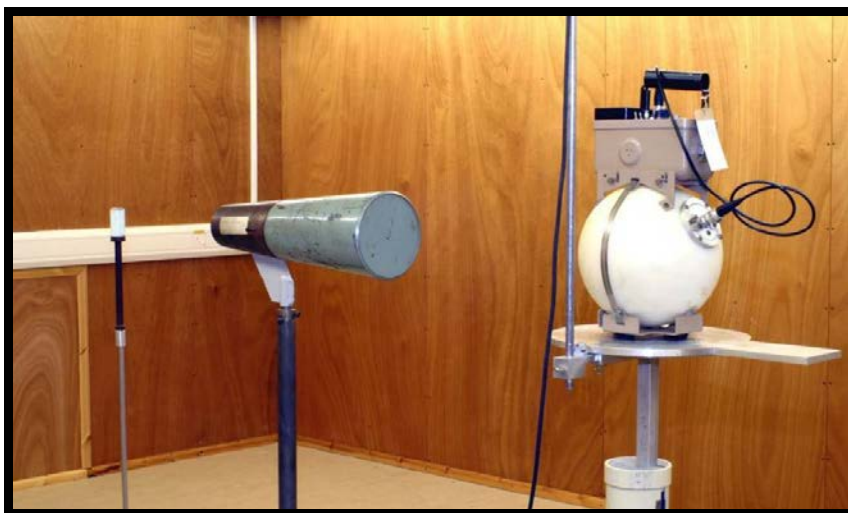
FIGURE 1 Shadow cone set up in the Neutron Laboratory at PHE
