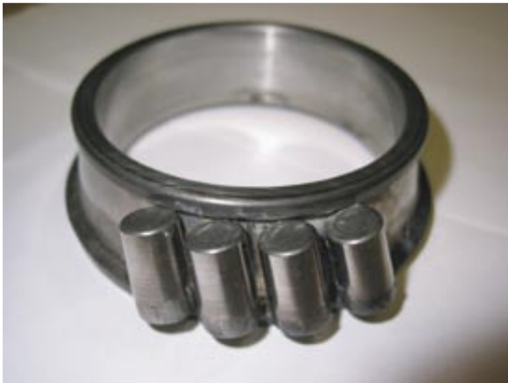
Figure 6 (left) Rollers welded to cone
