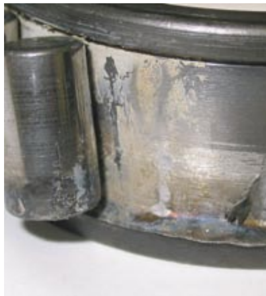
Figure 7 (right) Distortion of cone large rib face
