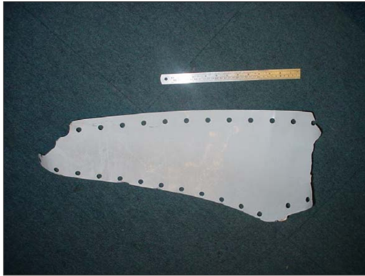
Section of outer skin of right engine pylon panel 427AL found on the runway
