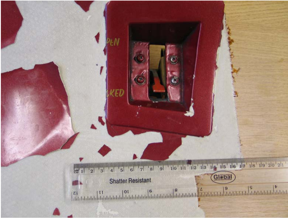
Figure 1 - Engine cowling - Aft latch (outside) and latch lever
