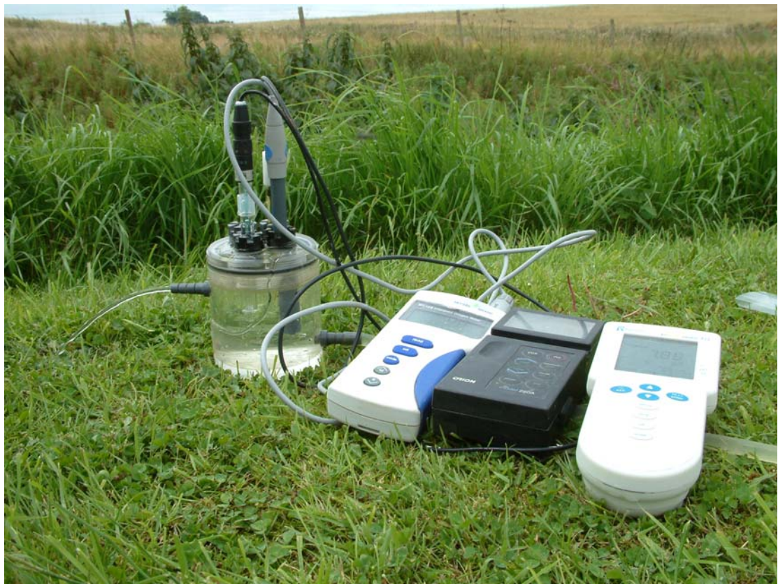
Figure 4.4 Unstable parameters are sampled using a flow through cell
