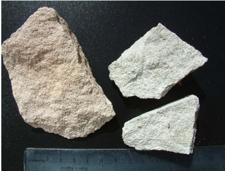
Figure 3.3 Samples showing differences in colour in the Lincolnshire Limestone. The sample on the left hand side is of the more oxidised buff coloured limestone where as the samples on the right hand side are less oxidised and grey in colour. All samples are from Metheringham Quarry.
