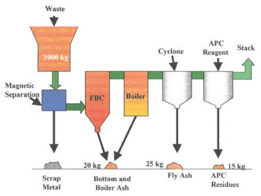
Figure 6 Waste residue streams for a fluidised bed incinerator (Source: Energy from Waste Association, 2000)
