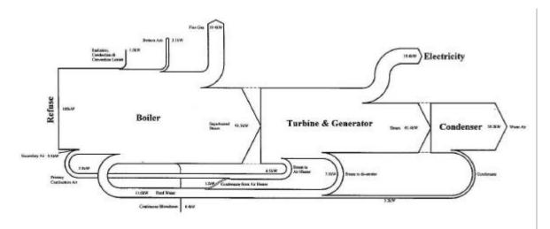
Figure 8 Energy flows of a model waste to energy facility
