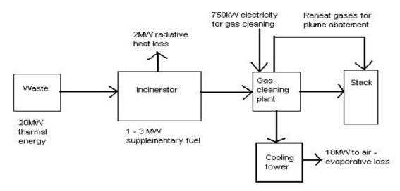
Figure 9 Energy flows within a hazardous waste incinerator (Source: Shanks 2001)
