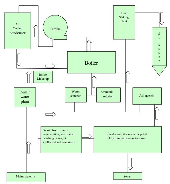
Figure 3 Water cycle for a typical mass burn waste to energy facility (Source: SELCHP 2001)
