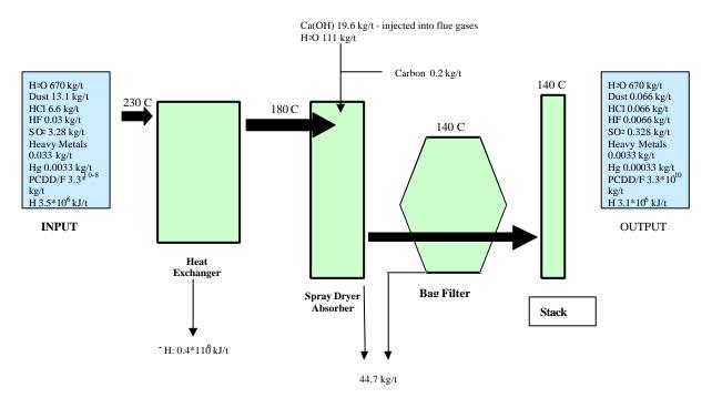
Figure 1 Schematic of inputs and outputs for semi-dry abatement plant
