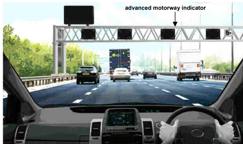
Figure 4A: Illustrative M1 J28 to J31 managed motorway scheme section operating in normal motorway conditions with blank advanced motorway indicators and blank gantry mounted variable message sign
