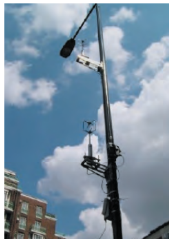
Figure 3: Two ultrasonic anemometers mounted on a lamppost. These instruments measure the three components of the mean wind and turbulence. Also mounted on the lamppost and visible towards the bottom of the picture is the instrumentation for measuring carbon monoxide (CO) concentrations.
