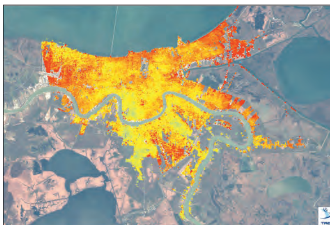
Figure 6: PSI subsidence image of New Orleans for the 3 years before hurricane Katrina struck in 2005. Yellow areas are subsiding at 5mm/yr and red ones at 10mm/yr or greater (Courtesy: TRE and Miami University).
