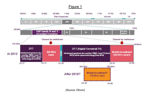
The diagram sets out the allocation of spectrum relative to frequency. The frequency range for the UHF band is 300MHz – 3GHz (3000MHz) and referred to as the 'sweet spot'. The UHF bands IV and V are of particularly high commercial value compared to the rest of spectrum and therefore of particular focus for this impact assessment. The range has an ideal combination of data transfer rate and distance the data can travel, thereby characterised by high market demand and relative scarcity.
