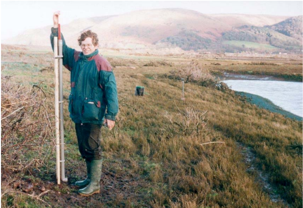
Figure 29. Extreme water level recorder sited on the margin of the lagoon close to MHWST. The water sensitive tape is attached to a rod that is held vertically within the standpipe. Water can only enter at the base of the standpipe and dissolves the dye of the tape as the lagoon level rises. The rod and tape are withdrawn from the pipe for measurement and a fresh tape is attached to the rod following each measurement. The standpipe is weatherproof so preventing entry of water except as the lagoon level rises.
