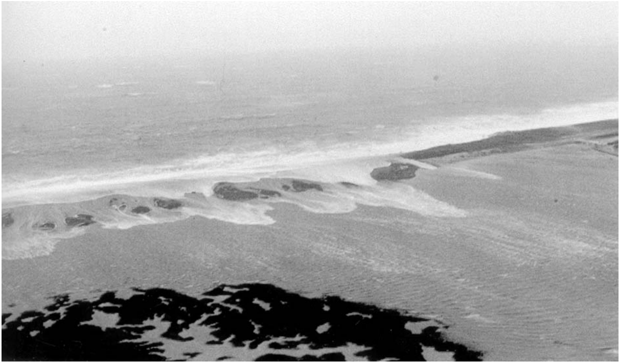
Figure 8. Overwashing in progress on Hurst Spit, Hampshire on 18.12.89 (photo courtesy of Dr Andrew Bradbury). Similar processes occur at Porlock and would have initiated the 1996 breach.
