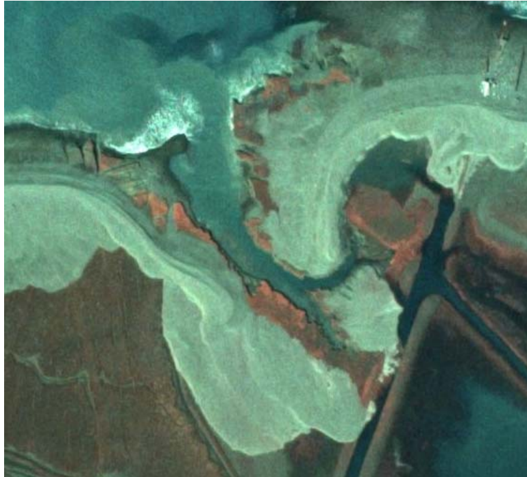
Figure 16. Near-infrared digital image of the breach approaching high tide at 1345hrs (GMT) on 4 th September 1999. Note that the tide has yet to rise above the clay cliffs and platform and that the two “waterfalls” have retreated closer towards the main artificial drainage cut. Gravel entering the incised channel has formed a small temporary spit on the western flank. This imagery is especially effective for study of vegetation. Algae on the clay platform show up bright red and saltmarsh is darker (bottom left). Waters around the breach are turbid due to wave erosion of the clay cliffs.
