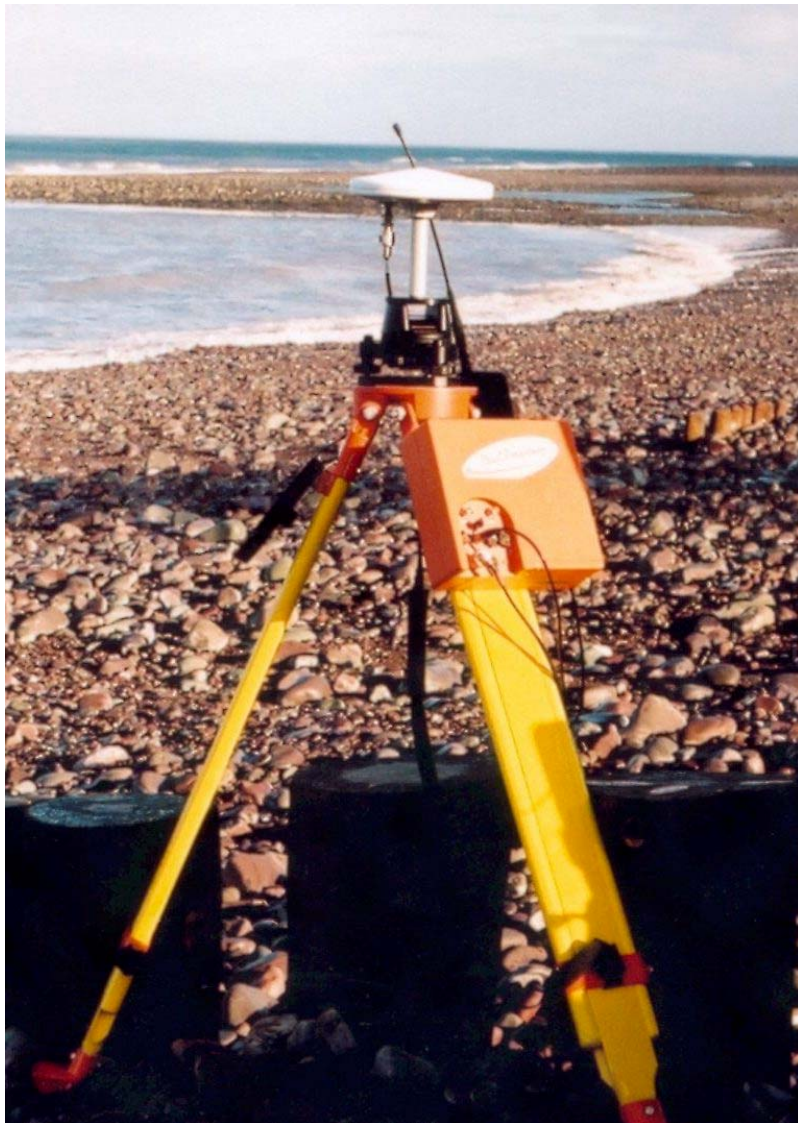
Figure 23 GPS survey equipment in operation. A static receiver is set up at a known point and the surveyor operates a roving receiver measuring profiles and other features of detail to complete the survey. Note that a radio link operates between the two enabling the surveyor to measure all points in real time.
