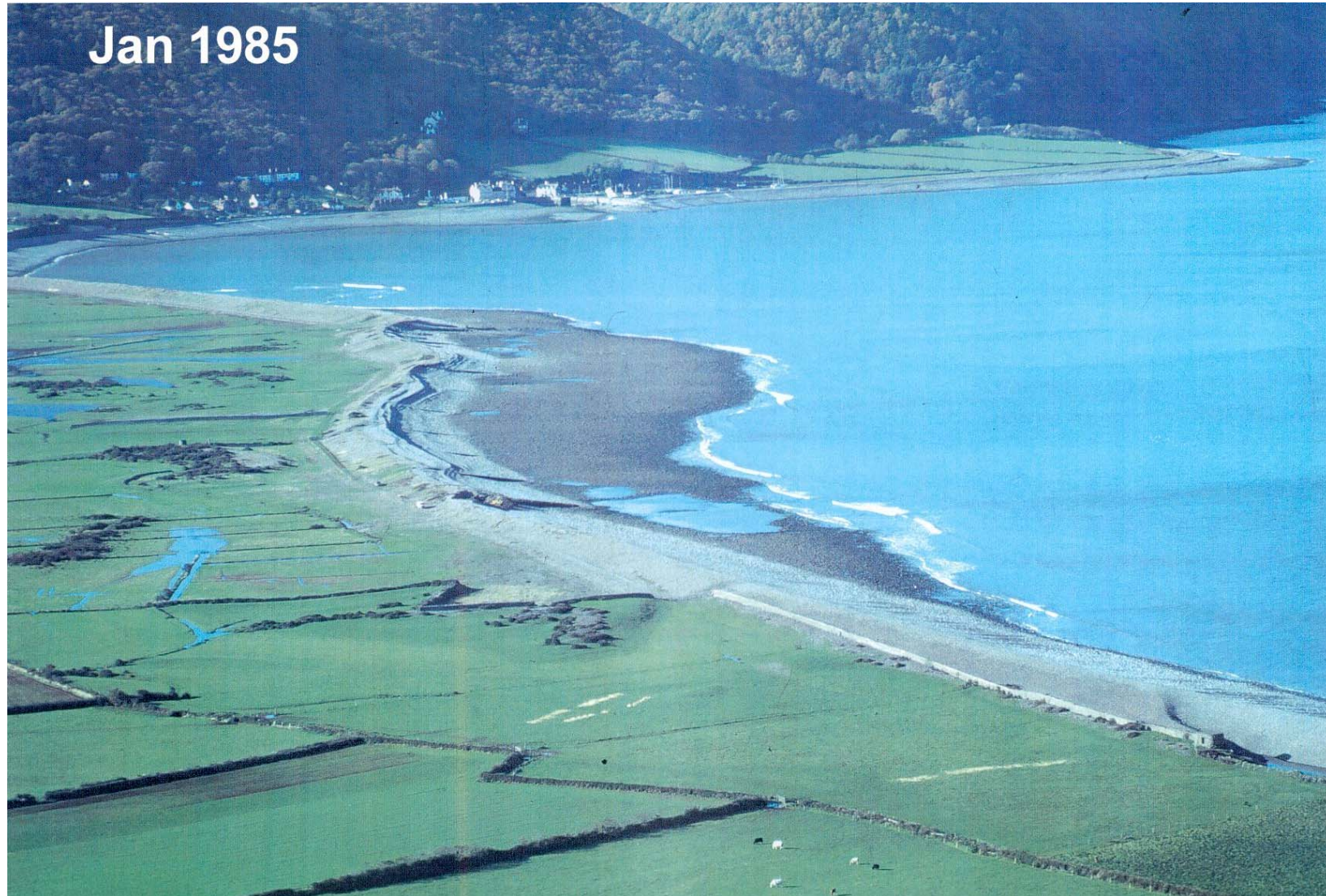
Figure 3 View westwards across Central Parts of Porlock Bay demonstrating the artificially maintained barrier with its steep and high crest. During this time, the back-barrier area was a freshwater grazing marsh drained by the sluice at New Works (mid distance). The exposed foreshore represents land transgressed by the retreating barrier.
