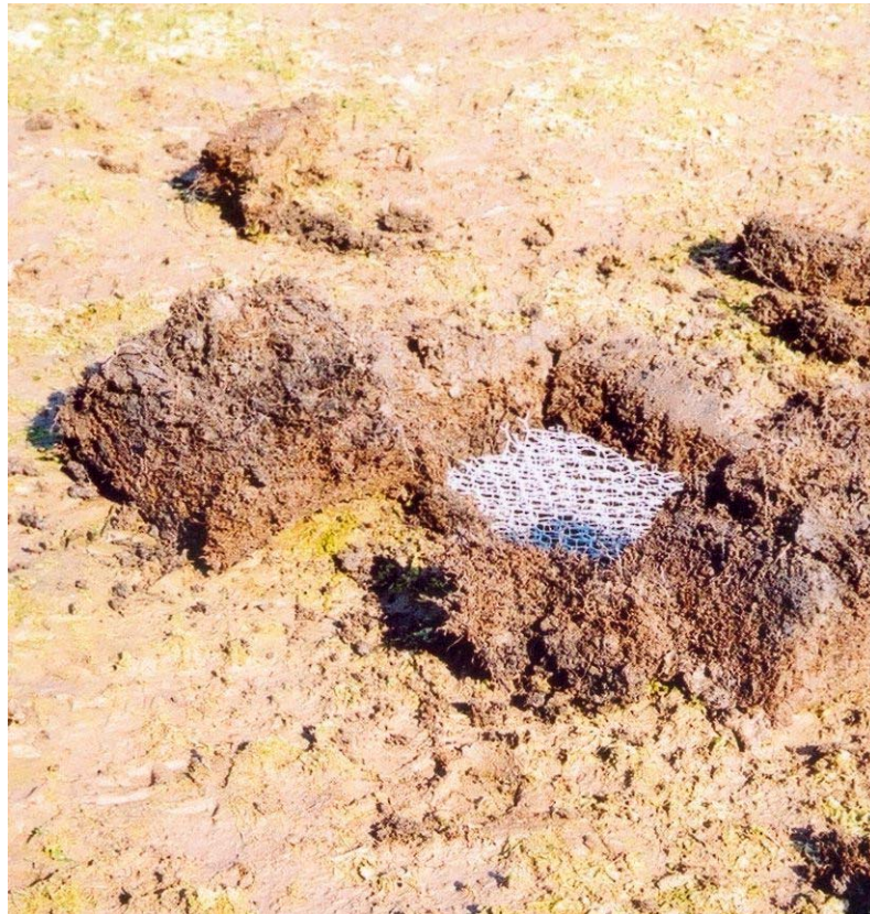
Figure 33 Insertion of accretion plate B (mid lagoon margin) at accretion profile E2. The wire mesh was buried carefully at 100mm depth by replacing the marsh turf to minimise disturbance. The site is relocated using a metal detector to pin point the wire mesh. To measure accretion a steel rule is pressed into the marsh surface until it encounters the wire mesh.
