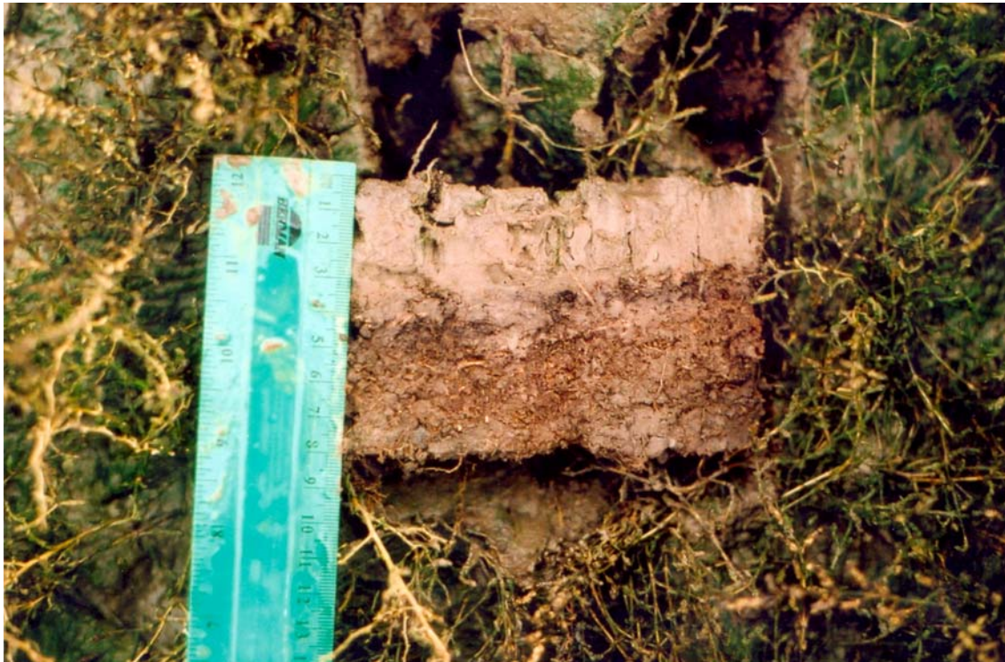
Figure 35. Turf cut from profile E2 upper site showing the clearly defined 30-40mm thick clay layer above a former vegetation/soil surface. This is believed to represent the thickness of marine accretion that has occurred following the breach in October 1996.
