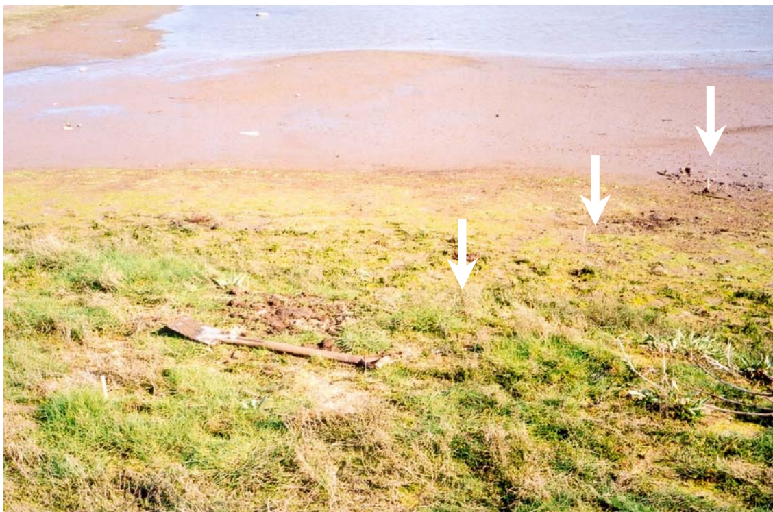
Figure 34 Accretion profile E1 at the lagoon margin. Arrows indicate the locations of the buried accretion plates. The aim is to record accretion occurring at different elevations and with different levels of vegetation cover.
