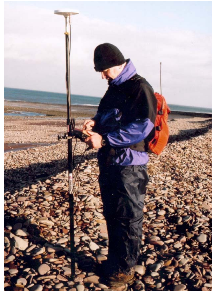
Figure 23 GPS survey equipment in operation. A static receiver is set up at a known point and the surveyor operates a roving receiver measuring profiles and other features of detail to complete the survey. Note that a radio link operates between the two enabling the surveyor to measure all points in real time.
