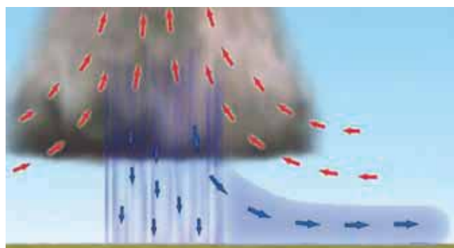
Figure 1: Schematic profile of airflow in a thunderstorm © Met Office
