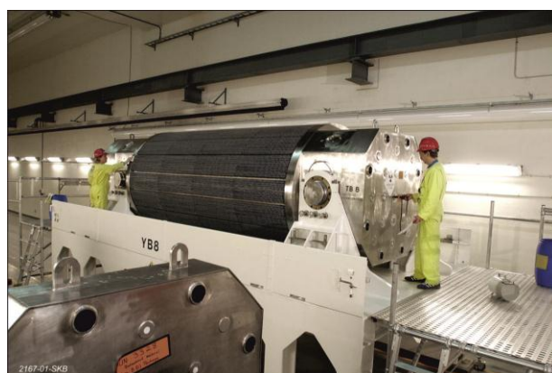
Receipt of HLW transport cask at CLAB (central underground interim storage facility for spent nuclear fuel), Sweden (courtesy SKB)
