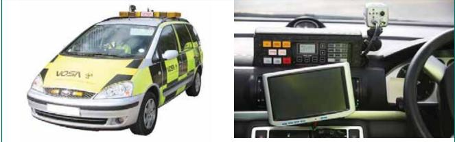
VOSA enforcement vehicles are equipped with ANPR cameras and other innovative mobile technology to help us target the non-compliant.
