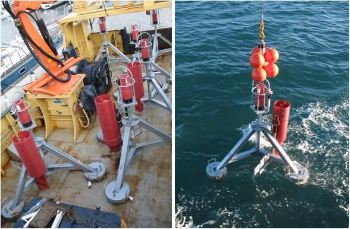
Figure 4. Left, VR3 equipped landers aboard Plymouth Quest and right, being deployed at the test site in Whitsand Bay, Cornwall.
