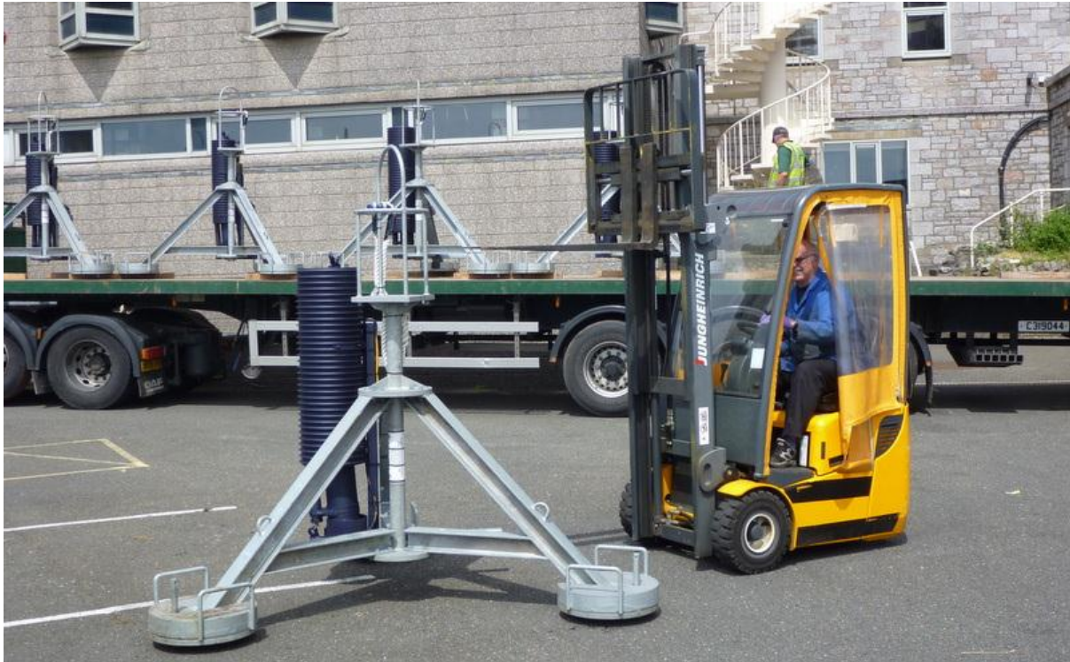
Figure 6. Loading 6 completed landers (minus the VR3 fish tracking and recording device) on to the lorry at the MBA. The blue parts are the antifouled release and recovery mechanism, which at this time have the anti-vibration foam blocks inserted.
