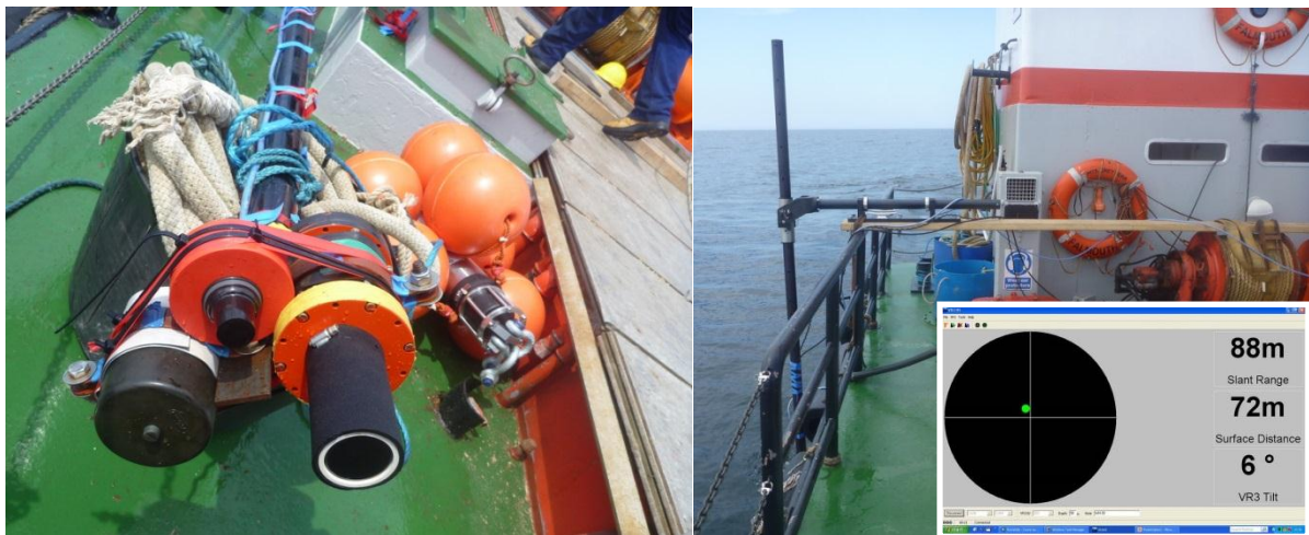
Figure 7. Left, the three dunker units for the IXSEA 2500, the Sonordyne lightweight release transponder and the Link-Quest modem for the VR3. Also visible is the IXSEA 2500 and its supplementary flotation. Right, the MBA's GeoAcoustics survey pole and mount in position. Inset is a screenshot of the VR3 host software, used to verify the location and attitude of the lander during deployment and once on the sea bottom. This one shows the tilt on lander 3 at the southwest corner of the Wave Hub Deployment Area, which had the greatest tilt angle of all those deployed at Wave Hub.
