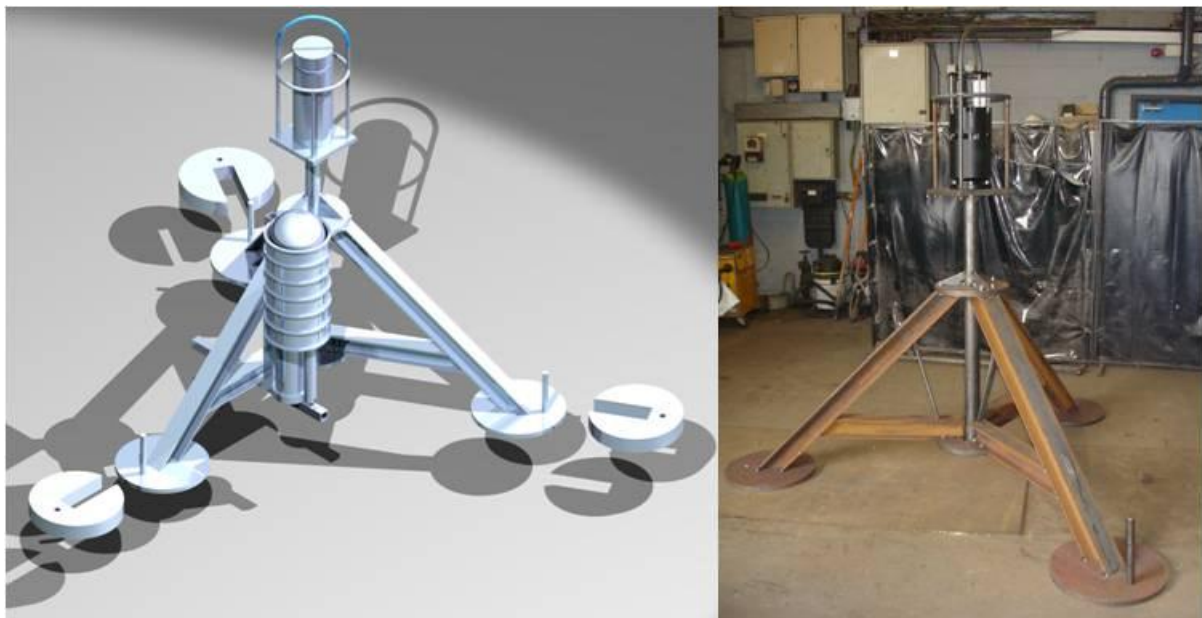
Figure 3. Left, completed, rendered PowerSHAPE-e CAD image of lander and additional foot weights and right, the tack-welded prototype.
