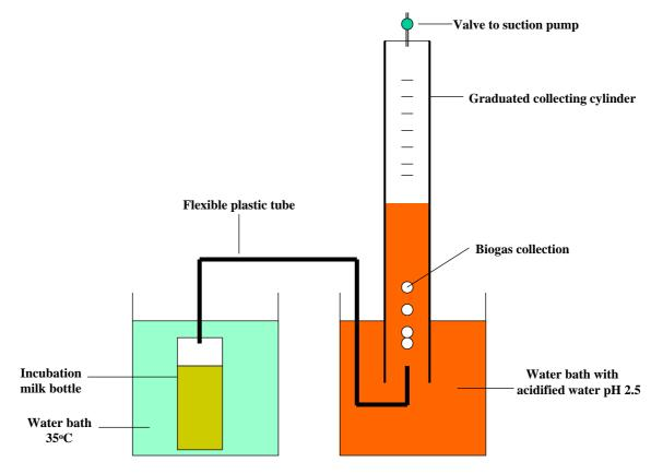
Figure A.1 Schematic of BM100 method set up.
