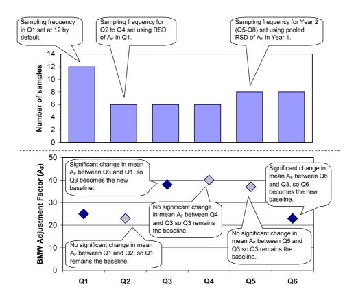
Figure 6.3 Example showing how to determine the required sampling frequency and assess the performance of the plant using change in  $A_f$ .
