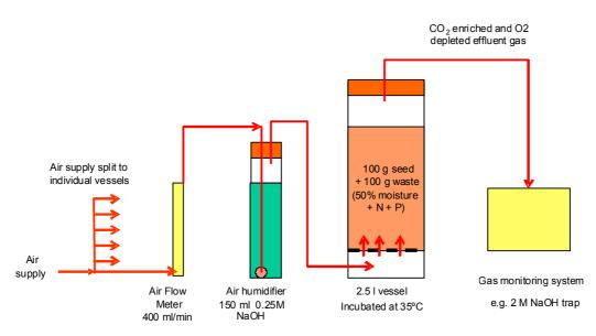
Figure A3 Schematic diagram of aerobic DR4 test set up
