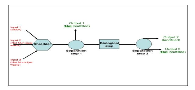
Figure 8.2 Example MBT with three inputs of which only one is municipal waste.
