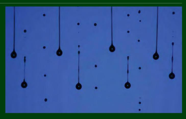
**Above:** This image captured with a very brief (20 ns) flash shows jets of ink ejected from an array of 11 nozzles at the top of the frame.*Credit: University of Cambridge, Inkjet Research Centre.*
