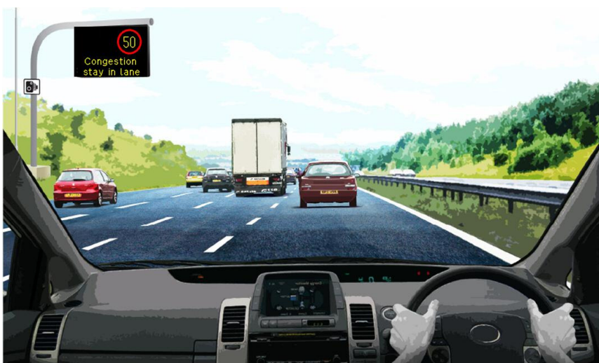
Figure 4D: Illustrative M1 J32 to J35a Managed Motorway scheme section operating with variable mandatory speed limits and information for road users.
