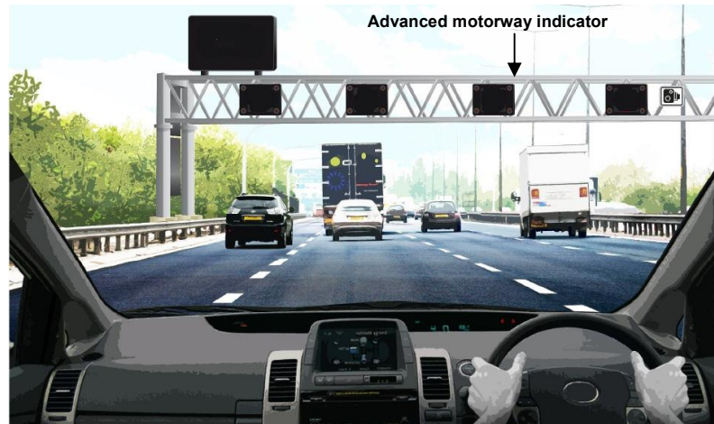
Figure 4A: Illustrative M1 J32 to J35a Managed Motorway scheme section operating in normal motorway conditions with blank advanced motorway indicators and blank gantry-mounted variable message sign
