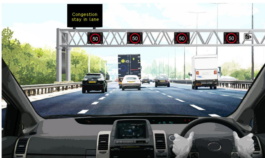
Figure 4C: Illustrative M1 J32 to J35a Managed Motorway scheme section operating with variable mandatory speed limits
