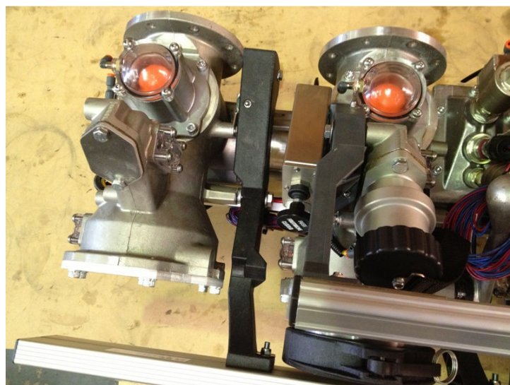
Figure 22 Auxiliary manifold section for loading operation
