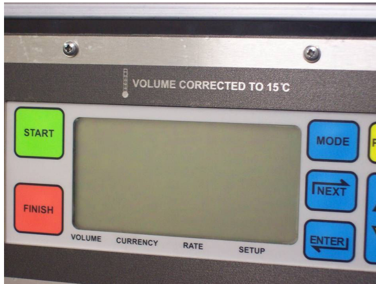
Figure 20 Typical legend showing temperature correction
