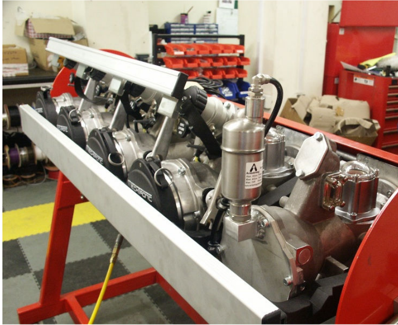
Figure 23 Auxiliary manifold section for drawbar tank trailer operation showing auxiliary air eliminator
