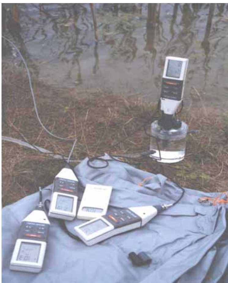
Figure 4.1 Unstable parameters are measured in an anaerobic throughflow cell.
