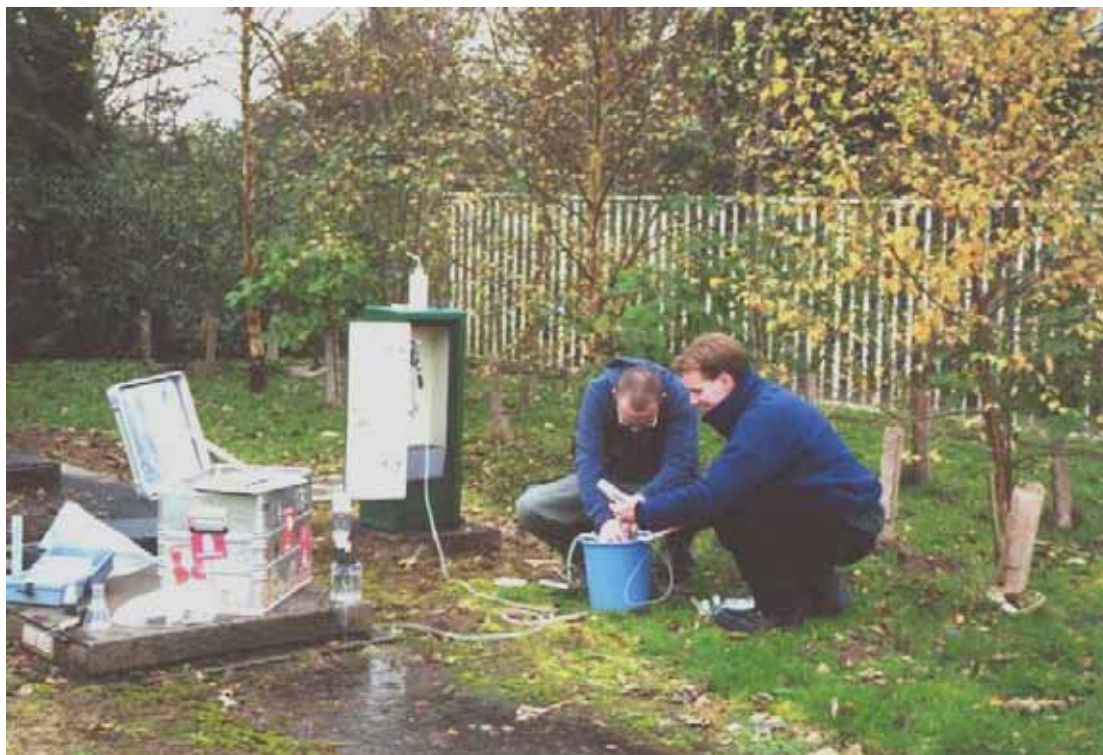
Figure 4.1 On-site sampling using a flow through cell .
