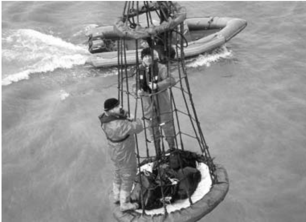
Figure 6.1. Example of a Billy Pugh personnel transfer basket
