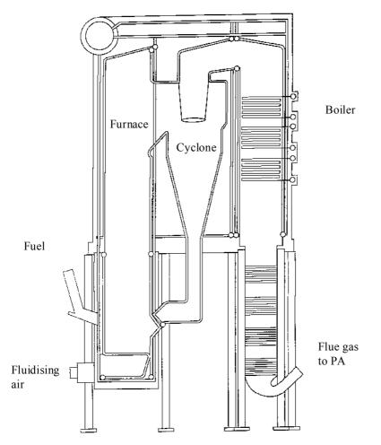
Figure 5.3 Schematic of circulating fluidised bed combustor
