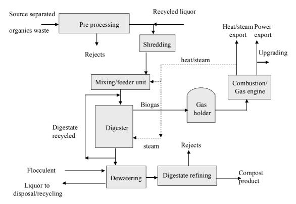
Figure 4.1 Anaerobic digestion process
