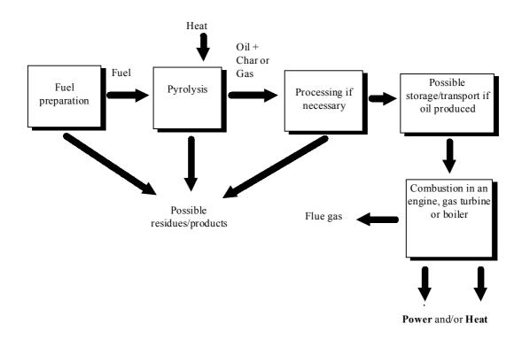
Figure 6.2 Schematic representation of pyrolysis process
