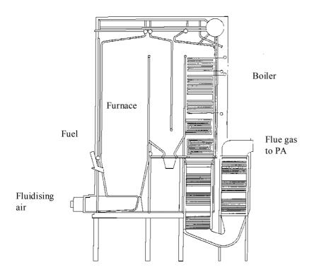
Figure 5.2 Schematic of bubbling fluidised bed combustor
