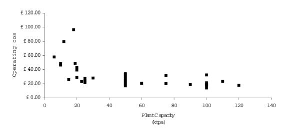
Figure 3.3 Gate fees for in-vessel composting systems in Europe (corrected to year 2000 basis)
