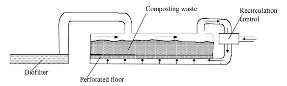
Figure 3.1 Schematic representation of batch tunnel composting
