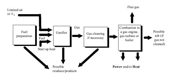
Figure 6.1 Schematic representation of the gasification process
