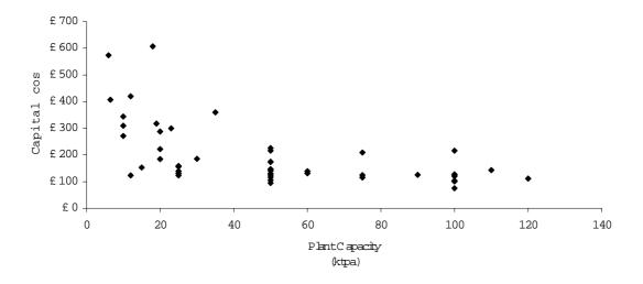
Figure 3.2 Capital costs of in-vessel composting systems in Europe (corrected to year 2000 basis)
