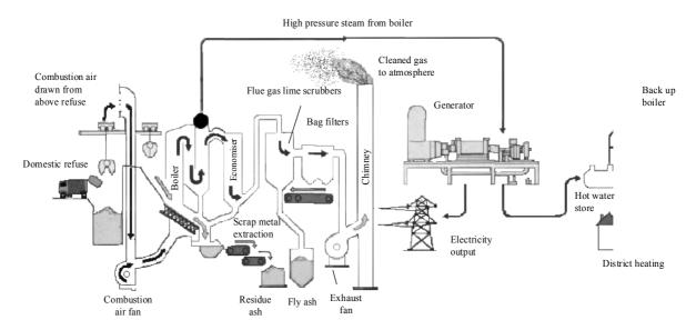
Figure 5.1 Typical mass burn incineration plant
