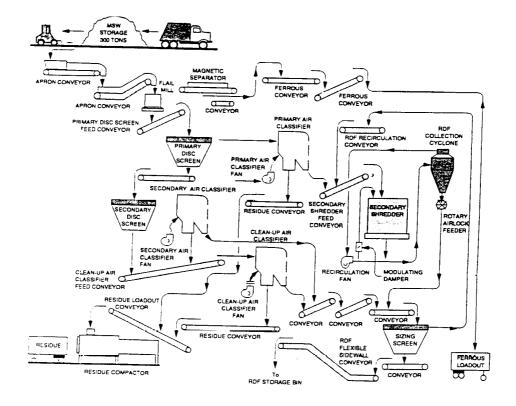
Figure 5.5 Flowline for floc RDF production at NSP French Island
