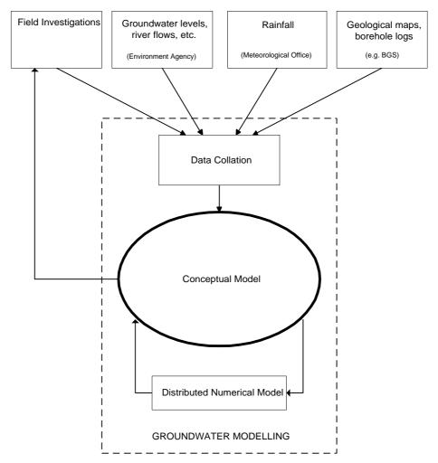
Figure 3.1 An overview of the groundwater modelling process
