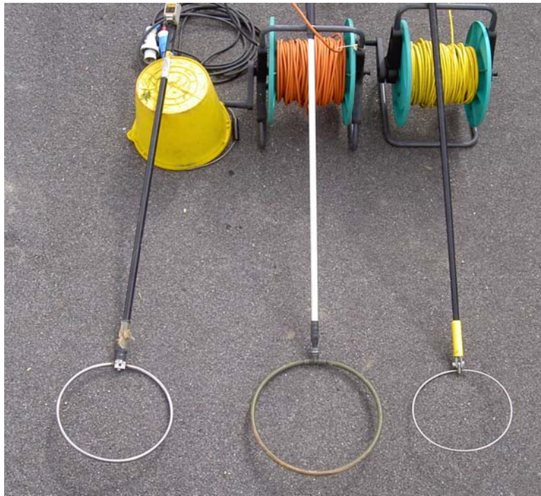
Figure 3 Pulse box manufacturers anode designs. Left to right, Electracatch; Millstream; Intelysis
