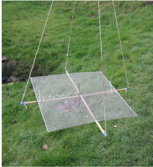
Figure 4 Mesh design cathode suspended in non-conducting cradle
