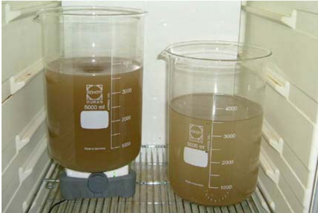
Plate 3.4: Stirred (left) and settled (right) microcosms within incubator at end of six hour experimental period (note the difference in turbidity between the two microcosms)
