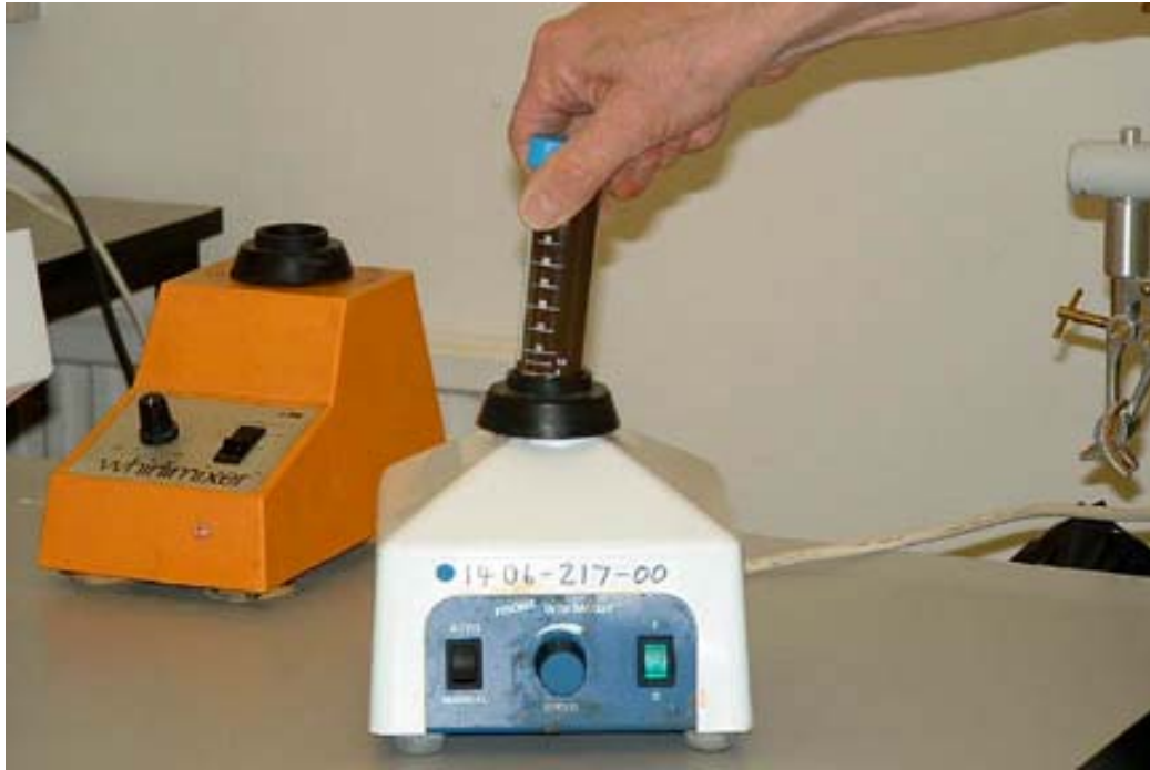
Plate 3.2: Vortexer (Fisons Whirlimixer) used in the experiments to determine the optimum method for separating enterococci from sediments
