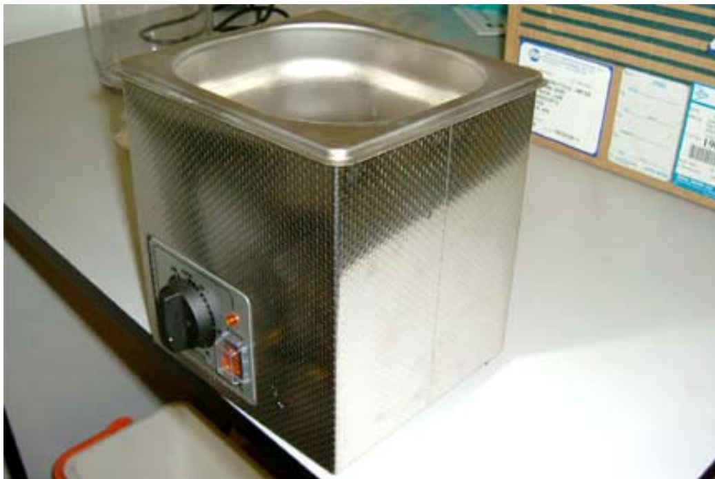
Plate 3.3: Ultrasonic bath (Ultrawave Model No. M12140) used in the experiments to determine the optimum method for separating enterococci from sediments
