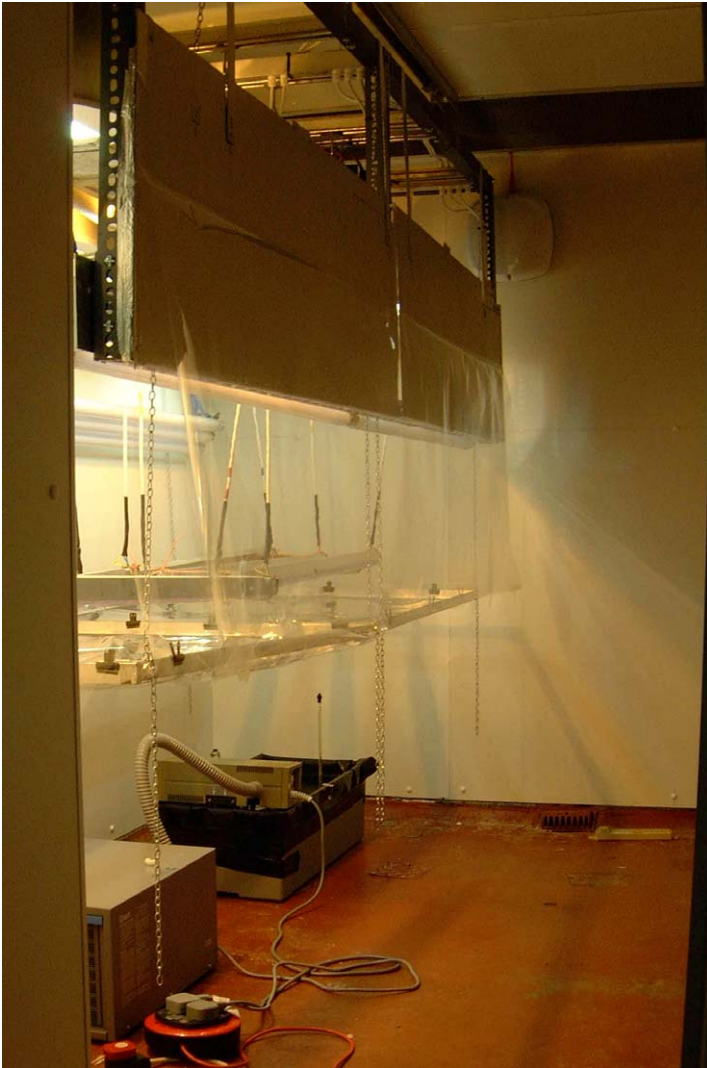
Plate 2.1 (left): Irradiated microcosm in-situ beneath artificial light source
