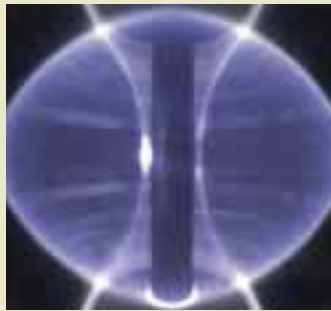
Controlling the large balls of plasma inside full-size fusion reactors is one of the challenges facing scientists. Shown here is a three metre diameter plasma ball inside MAST, the UK's own fusion device.
