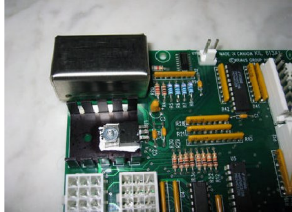
Figure 5 Cover enclosing the dip switches and the two trimmers
