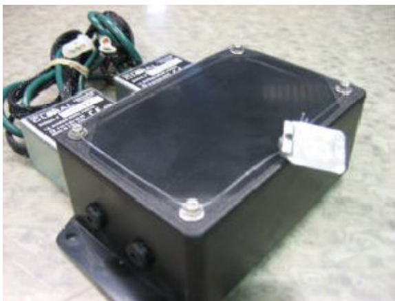
Figure 6 Securing of I.S. barriers
