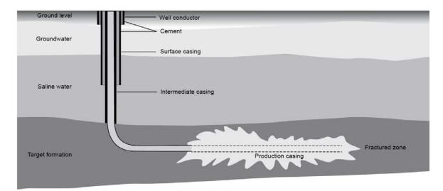
Figure 2.2 Schematic of a horizontal well
