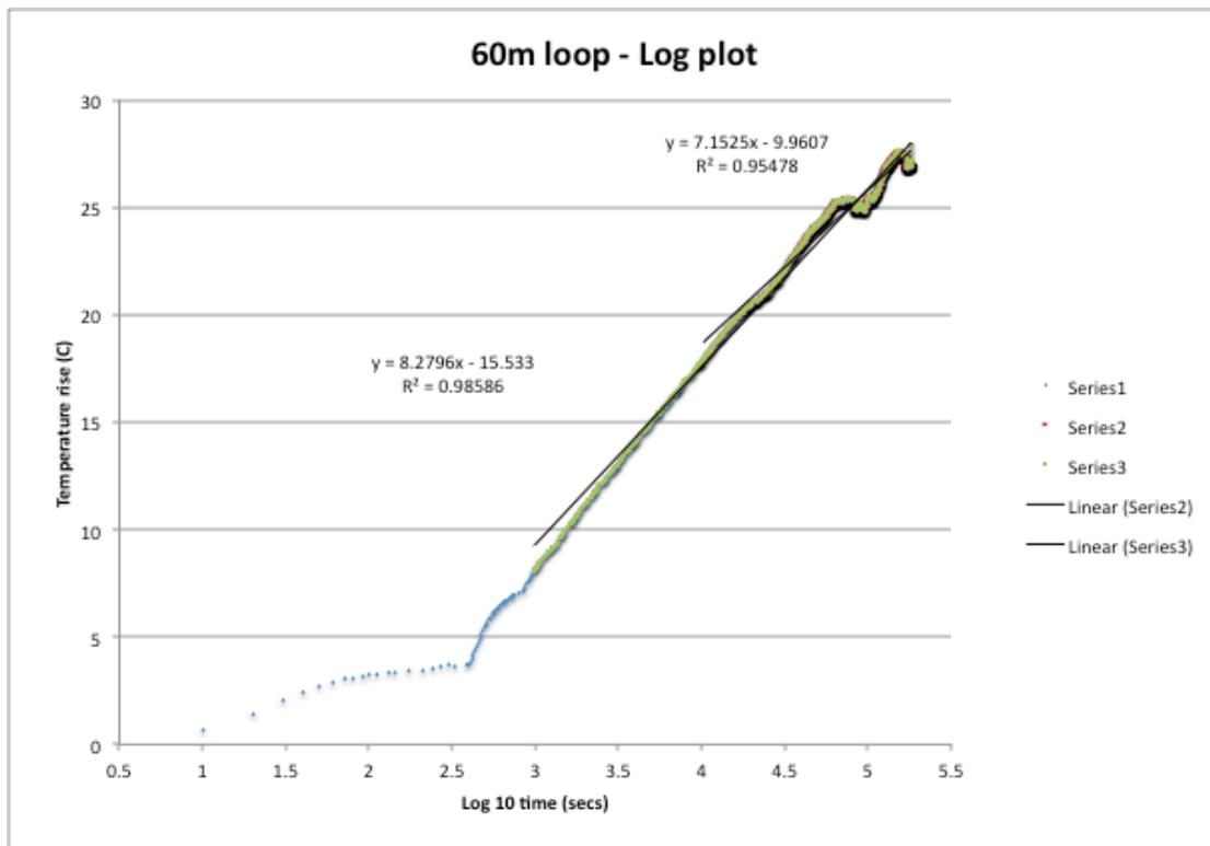
Figure 9: Log plot of temperature increase for 60m test.
