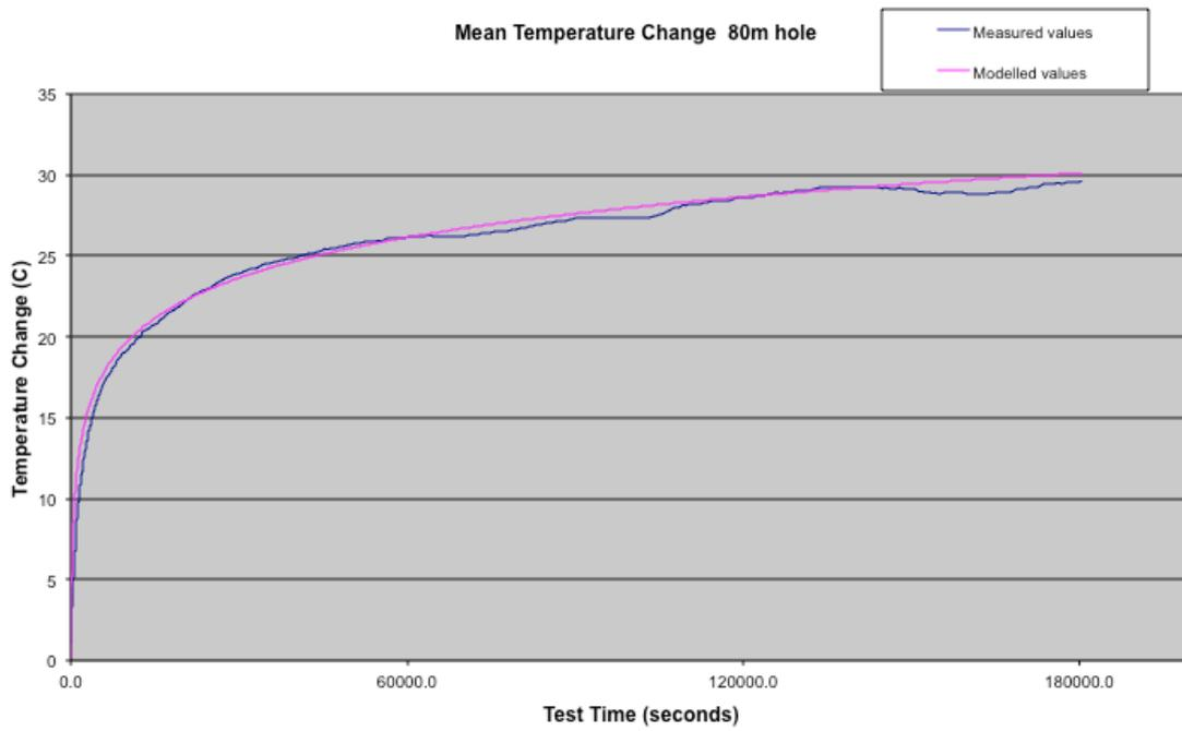
Figure 10: Analytical solution used to match 80m thermal response test.
