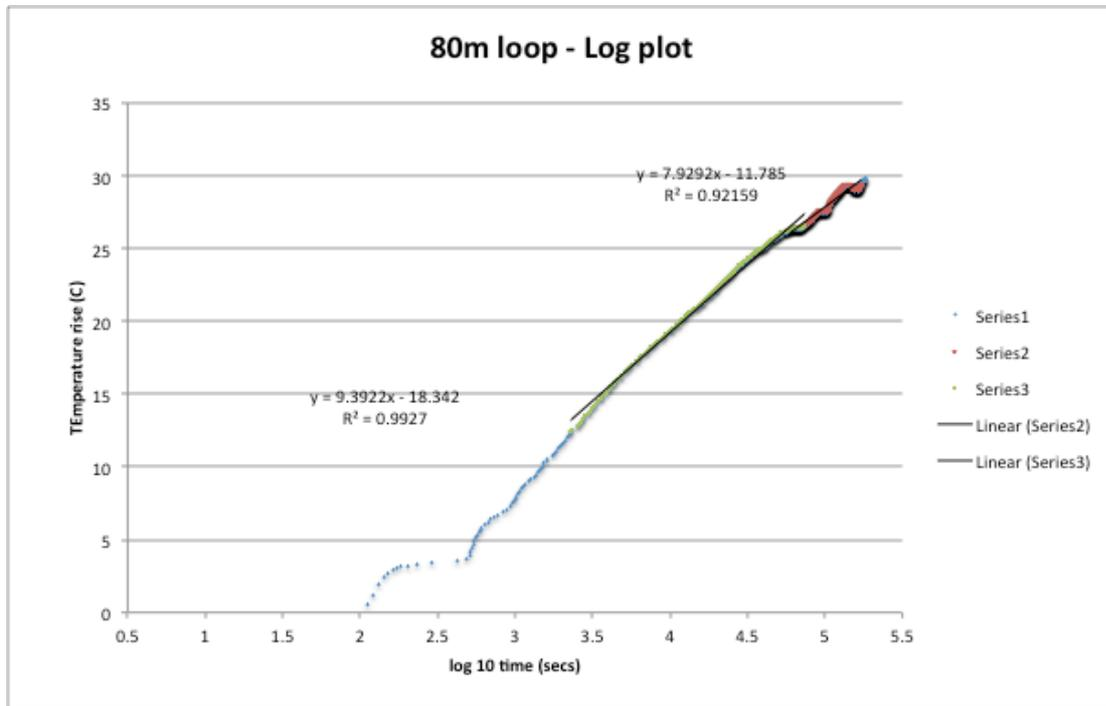
Figure 8: Log plot of temperature increase for 80m test.
