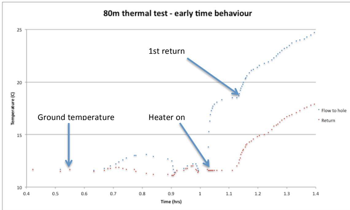
Figure 6: Early time behaviour of 80m thermal test.
