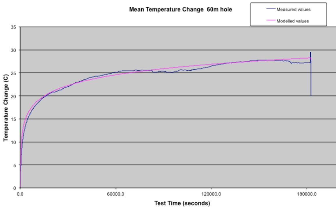
Figure 11: Analytical solution used to match 60m thermal response test.
