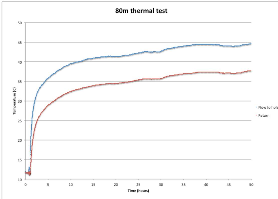
Figure 4: Flow and return temperature profile of 50 hour test on 80m borehole.
