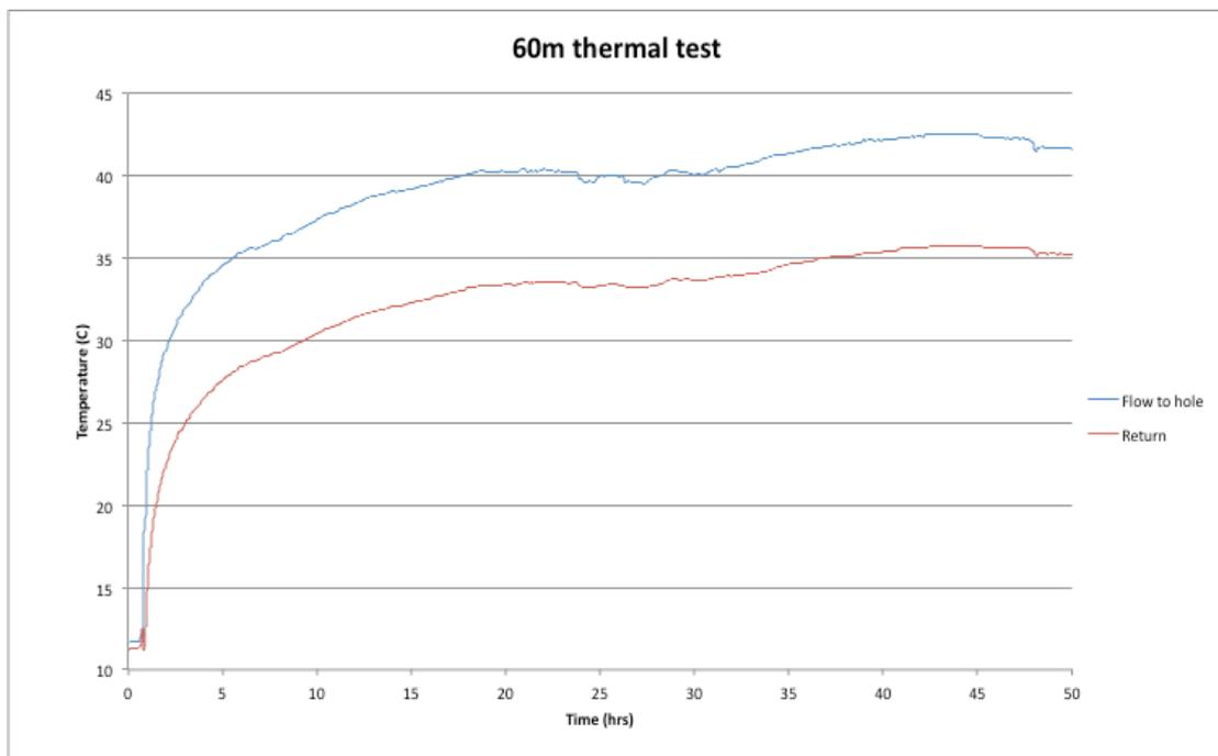
Figure 5: Flow and return temperature profile of 50 hour test on 60m borehole
