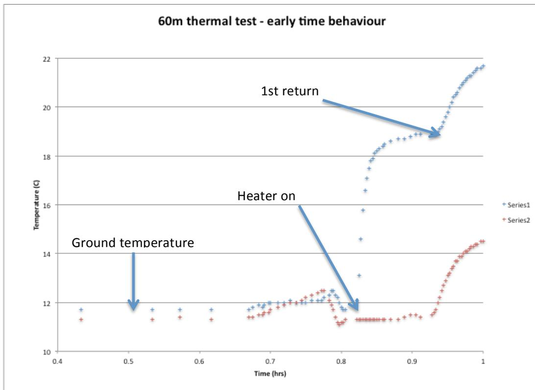
Figure 7: Early time behaviour of 60 m thermal test.
