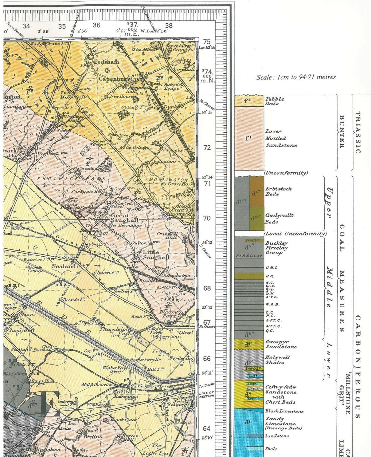
Figure 3: Extract and key from relevant solid geology map of the site. (see top right).
