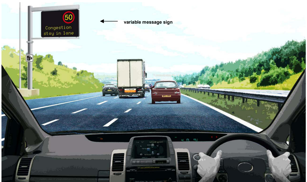
Figure 4D: Illustrative VMSL scheme section operating with variable mandatory speed limits and information for road users.
