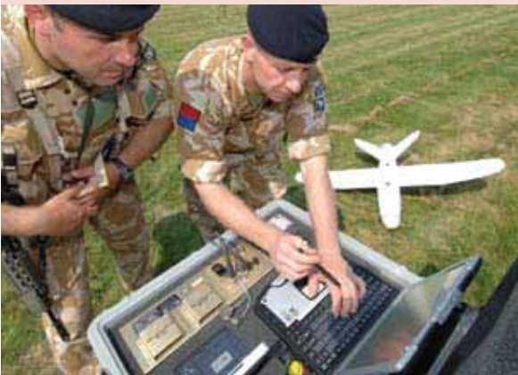
The Royal Artillery getting to grips with the Ground Control System for the new UAV “Desert Hawk” before they deploy to Afghanistan
