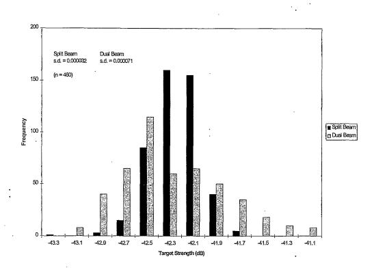
Figure 2.3: Target strength measurements of a tungsten carbide sphere using the dual-beam and split-beam techniques (Traynor and Ehrenberg, 1990).
