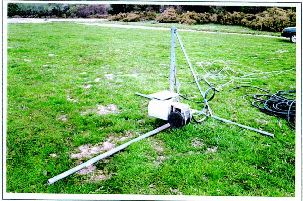
The transducer mount designed for the River Spey. Figure 3.5: Photographs of two types of temporary transducer mount.
