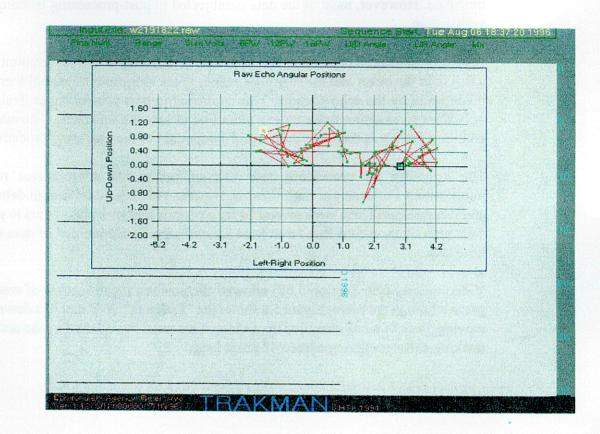
Figure 5.8: TRAKMAN screen showing an X - Y plot of downstream moving weed that has been tracked by the automated tracking software.
