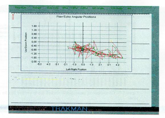
Figure 5.6: Example of a single fish trace that was broken up into several fish by the automated tracking software.
