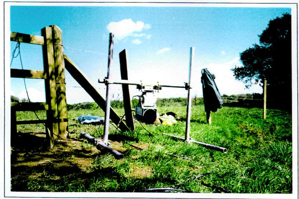
A temporary transducer mount used on the Wye.
