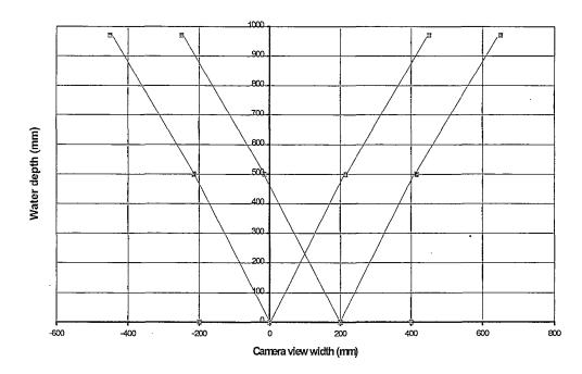
Figure 5.22: Video camera field of view.
