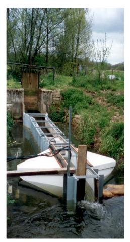
Plate 7.4 Video and resistivity smolt counting unit used to monitor smolt diverted into a bywash during BAFF<sup>™</sup> tests conducted by the Centre for Ecology and Hydrology (CEH) at the River Frome test site in Dorset.
