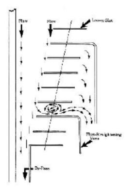
Figure 3.12 Schematic of louvre screen
