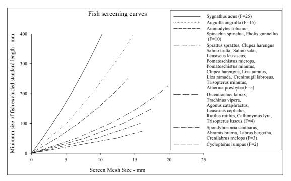
Figure 5.6 Mesh size curves for screening fish of different body shape, plotted from equation 1 (after Turnpenny, 1981, with additional coarse fish data from Table 5.1).
