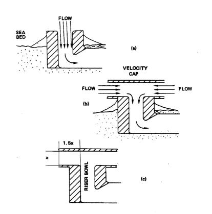
Figure 3.19 The velocity cap: (a) section of uncapped intake showing vertical draw-down pattern, (b) section of capped intake showing horizontal flow pattern, (c) as (b) but showing critical relationship between vertical opening [x] and length of horizontal entrance [1.5x] for fish reactions (after Schuler and Larson, 1975).
