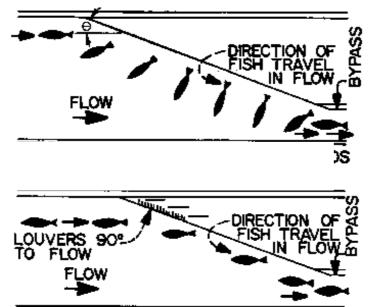
Figure 5.4 Fish movement in front of angled screens and louvres. Lower diagram applies when the channel velocity is below or near the maximum sustainable swimming speed of the fish, upper diagram when channel velocity exceeds the swimming speed of the fish (Rainey, 1985).
