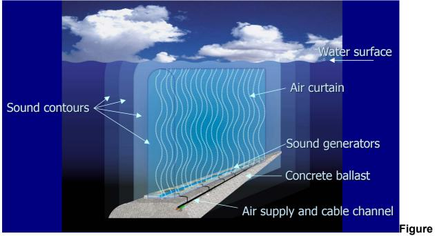
3.18 Schematic of BAFF<sup>™</sup> acoustic bubble curtain (Fish Guidance Systems Ltd)
