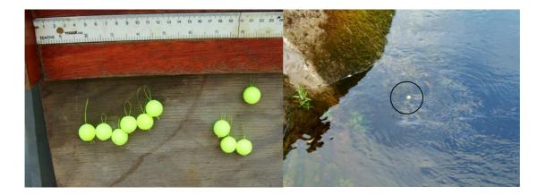
Plate 7.5 Fluorescent polystyrene float tags as used to follow close-range movements in front of screens and bywashes. The left-hand photograph shows a number of floats prior to attachment; the right hand side shows one as viewed in the water (inside black circle).
