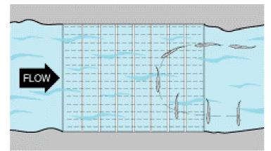
Figure 3.21 Diagram showing fish movement in response to the GFFB electric fish barrier. In the diagram, the energisation voltage of the electrode strips increases from right to left of the diagram. The fish turn away at a point depending on their length and hence the voltage received along the body (<u>www.smith-root.com</u>).
