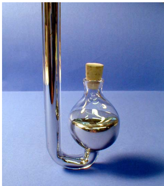
Photograph: Mercury 'cistern' type tube for a mercury barometer (Note that with the cork bung in place, this barometer would not read accurately, but would reduce the amount of mercury vapour produced) (Source: Medford Clock Shop 3 )
