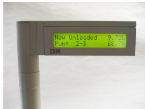
Figure 4 Customer display unit (CDU) illustrates transaction “A” & “B” on pump 2
