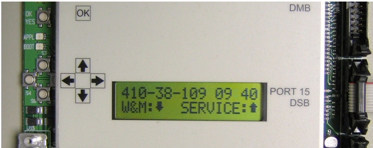
(c) Central Processing Board (CPB508) display and menu navigation keys
