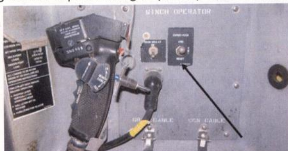
Fig 1-2 WOG in Stowed Position - Note Proximity of Arming Switch (Arrowed)
