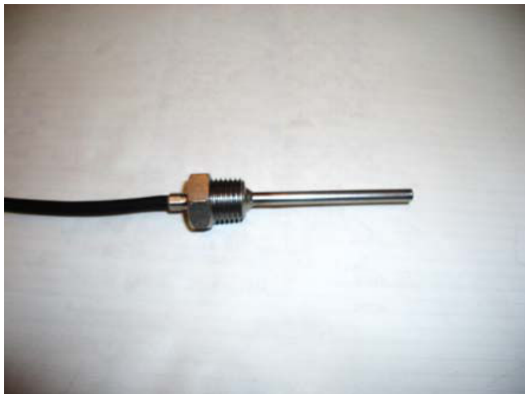
Figure 41 ATC Temperature Sensor
