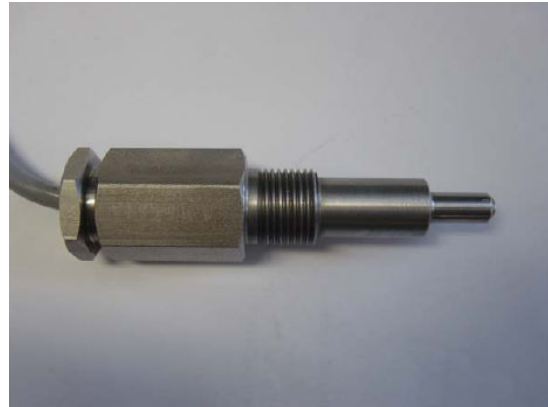
Figure 29 Temperature sensor: LM335
