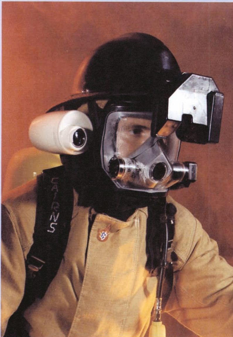
The helmet-mounted uncooled thermal imaging camera developed for the fire-fighting services by the DERA and GEC Marconi
